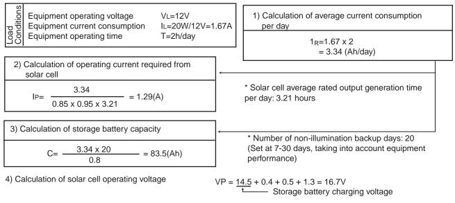
On the basis of the above, the most appropriate solar cell model is: the solar module BP-HK36K (Vp=16.7V, Ip=1.44A)
