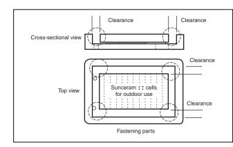
(4) The Sunceram II cells for outdoor use are provided with leads or solder electrodes on the rear, and these protrude. Grooves or holes should be provided in the area of the product where the cells are to be secured. The cells should be fastened in such a way that the leads or solder electrodes will not be brought into close contact with the fastening parts, thereby preventing distortion or deformation.
