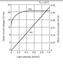
Open-circuit voltage, short-circuit current vs.
