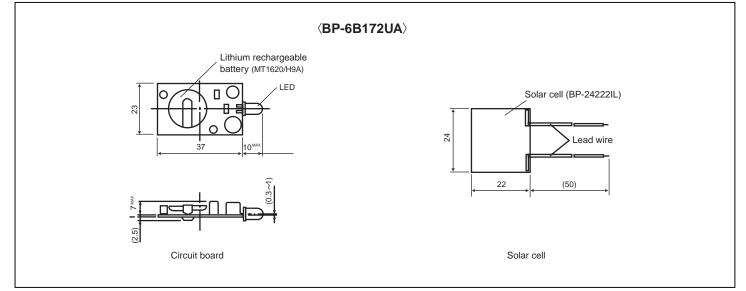
(Note) For detailed dimensions of the solar cell, refer to the Sunceram II Cell for Outdoor Use section.
