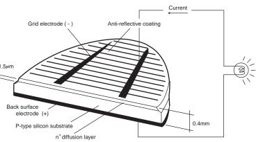
Electrons involved in forming the bonds between atoms fly out from the crystalline framework as free electrons bearing a negative charge. After the electrons have been given off, a positive electron hole is formed. An electrical field builds up inside the silicon present at the P-N junction and the electrons are scattered to the Ntype silicon. A voltage is produced at both electrodes and, if a load is connected to them, electrical power is supplied to it.
